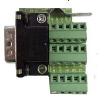
The terminals on the SM-ETC are labeled for a standard Quadrature Incremental Differential encoder with commutation channels. These labels will not match up with the wiring for a Stegmann Sin/Cos Absolute Hiperface encoder. The figure below shows the cross-reference.
